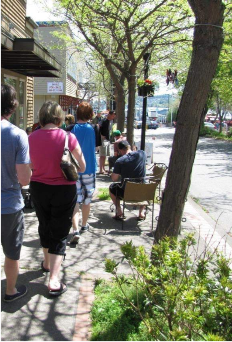
Figure 4.2 Illustration of height to width ratios that create a scale on thoroughfares that is comfortable to people and encourages walking (human scale). Human scale ratios fall between 1:3 and 1:2 as measured from the building fronts. Source: Community, Design + Architecture.
